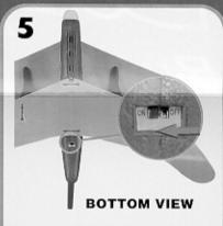
Turn on the plane by turning the Power ON/OFF switch to ON.
