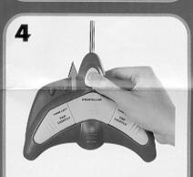
. Turn on the controller by pushing the Power ON/OFF switch up. The red ON/OFF indicator should light up when the controller is in use.
