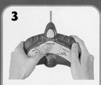
Press the PROPELLER ON/OFF button ONCE to start propellers. FLYING
