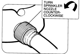
2. Fit the end of any standard garden hose into sprinkler nozzle. Turn sprinkler nozzle counterclockwise as shown to tighten. Turn on water to activate sprinkler.
