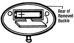
B. Unlatch door and tilt it down. Remove battery.
