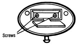
C. With a phillips screwdriver, remove only the 2 screws inside the battery compartment. This will allow removal of the bulb cover. A "bulb guard" will fall inside of bulb cover when screws are removed.
