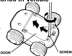
2. Insert 4 fresh "AA" batteries into compartment as shown. Replace battery compartment door, snap it back into place, and replace screw.
