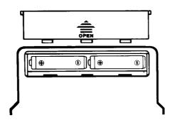
Insert two AA batteries, UM-3 or equivalent making sure to align "+" and "—" as shown.
