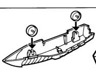
Wheels need to be snapped into place on both sides to allow boat to roll.
