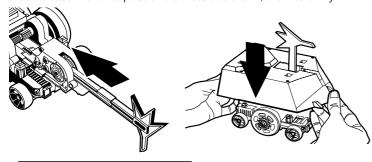
**NOTE:** Your **BattleBot** has a failsafe system. It will not operate unless the attachment is FULLY inserted.
