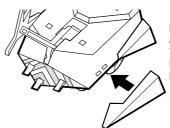
Finally, add the Bot's ablative defenses by attaching them to the body shell as shown. These pieces are designed to absorb impact and fly apart when the Bot is struck in combat.
