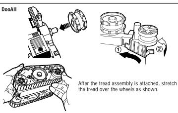
After the drive system is assembled, you can attach the Bot's offenses. Simply slide the attachment into place on the chassis as shown, and insert fully.
