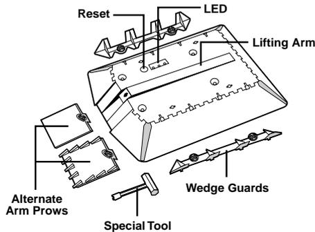
Use the special tool included with your **Pro Series BattleBot** to loosen or tighten the fasteners with a half-twist.
