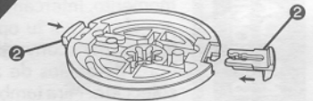
Insert Attachments (2) into Blade Base until the tips are just past the knobs. Do not insert attachments all the way in at this time.
