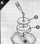
Assemble and attach spin gear parts (2) and (3) to Blade Base with screw. Note: Make sure screw is completely attached.
