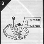
Place metal balls in Blade Base, starting with larger hole.
