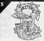
Attach the body, aligning the 4 screw holes to the posts.
