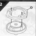
Place **()** Weight Disk on Blade Base assembly.
