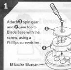
Note: Make sure screw is completely attached.
