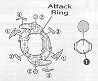
Place top ② on spin gear ③, and attach spin gear assembly to Blade Base ⑤ with the screw, using a Phillips screwdriver (not included).
