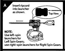
Insert posts on launcher into openings in BEYBLADE top, as shown.
