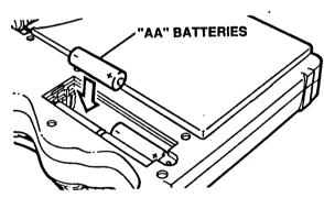
2) Place 4 "AA" size alkaline batteries (not included) into the compartment as shown. Be sure to place the positive (+) and negative (-) ends of the batteries in their proper location. Replace battery compartment cover and reinsert screw.
