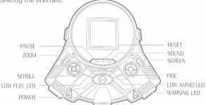
POWER — to turn the power ONOFF. (The unit also shuts off automatically after 3 minutes of inactivity.)
