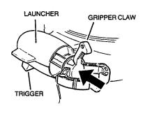
4) Fit one end of shock cord through hole in lower half of launcher. Tie a knot to secure. Repeat on other side.
