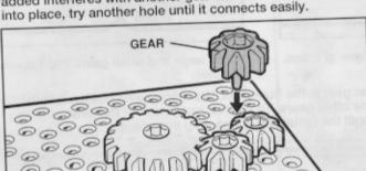
To spin the gears, place a crank handle into any large or small gear and start turning.
