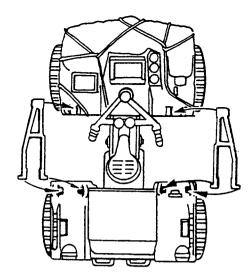
4. Attach safety gates at vehicle's sides in position as shown.
