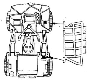
Insert post on stretcher into front hole, then back hole, as shown.
