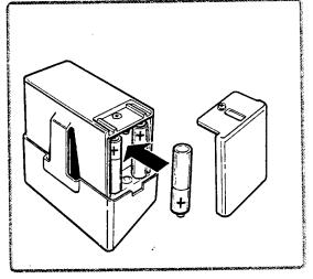
2. Insert 3 "AA" batteries (alkaline recommended), following direction indicators inside compartment. Replace door and tighten screw with screwdriver.
