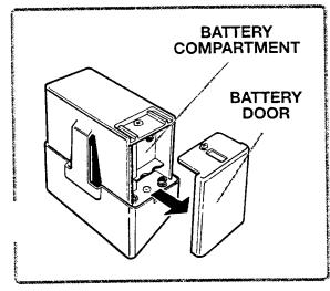
Locate the battery compartment on right bottom side of Power Pack. Use a Phillips screwdriver to loosen (but not remove) the screw that secures the battery compartment door, and remove door.
