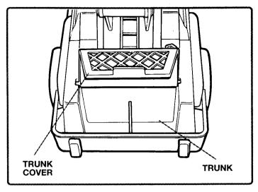
The trunk cover may be opened and closed to hold cargo in place.
