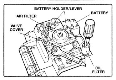
The Tow Truck's front cab opens up to reveal the engine. To lock and unlock the cab, there is a notch just below the driver's side door that can be opened with the screwdriver. Once you've opened the cab, use the wrench and the screwdriver to assemble the engine parts as shown: oil filter, valve cover and air filter. Slide battery holder/lever to secure battery in place.
