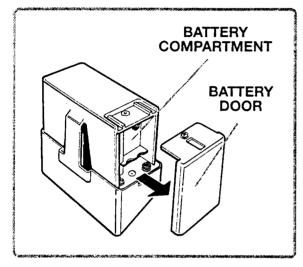
Locate the battery compartment on right bottom side of Power Pack. Use a Phillips screwdriver to loosen (but not remove) the screw that secures the battery compartment door, and remove door.
