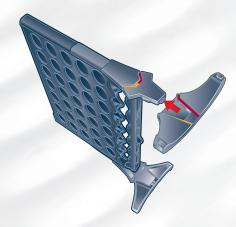
Attach feet to the sides of the grid.
