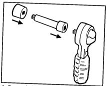
3. To reach those tight spots, fit the extender onto the handle, then the socket onto the end of the extender as shown.
