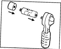
4. For maximum flexibility, fit the universal onto the handle, then the socket onto the end of the universal
