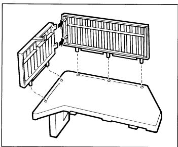
1. Fit the 2 railing pieces together, pressing the tabs on the long railing into the hooks on shorter railing. Then attach the assembled railing to deck, pushing the posts on railing into holes on deck.
