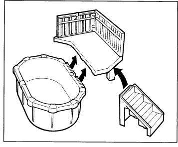
2. Assemble the deck to the pool as shown, fitting the deck into the 2 tabs in front of pool. Then add the stairs to the deck, again fitting the tab on stairs into bottom of deck.
