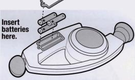
When to change the batteries: If BOP IT doesn't operate properly, or game performance changes, try reinserting the batteries. If that doesn't work, remove the old batteries, then insert three new batteries.
