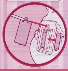
Use a Phillips/cross head screwdriver (not included) to loosen screw in battery compartment cover (screw remains attached to cover). Remove cover. Remove and discard old batteries. Replace with fresh 2 x 1.5V "AAA" or R03 size batteries. Alkaline batteries recommended. Replace cover and tighten screw.
