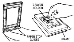
Place a sheet of paper under the frame firmly against paper stop guides. Rub the crayon holder softly against the paper in a circular motion.FOR THE BEST PICTURES, HOLD FRAME DOWN AND KEEP CRAYON LEVEL. The frame should also be cleaned periodically.
