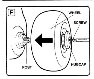
6. Place wheel on post. Place hubcap over post. Insert screw into hubcap and tighten with Phillips screwdriver. (See Illus. F.)
