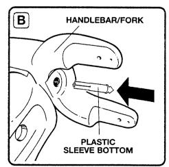
2. Turn toy on its side. Make sure bolt extends through hole in underside of handlebar/fork. Holding plastic sleeve top and bolt in place, slide plastic sleeve bottom over bolt and into hole in underside of handlebar/fork, (See Illus, B.)
