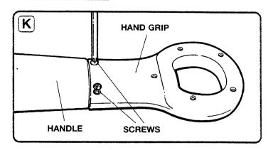
10. Slightly separate the two halves of the hand grip on the end. (See Illus. J.) Slide hand grip over top of handle. Align holes on end of hand grip with holes on end of handle, and insert 2 screws into holes. Tighten screws with Phillips screwdriver. (See Illus. K.)
