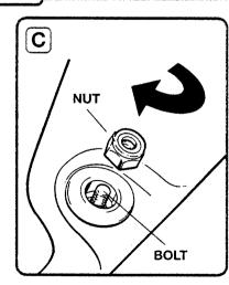
3. Place nut on end of bolt. Hold nut in place and tighten bolt with slotted screwdriver. (See Illus, C.)
