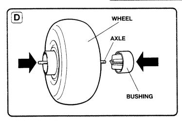
4. Turn toy upside down. Slide one bushing onto axle as shown. Slide wheel onto axle. Slide remaining bushing onto axle. (See Illus. D.)
