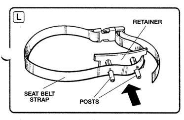
11. Insert posts on retainer through holes in seat belt strap. Make sure front of buckle will face toward you when fastened. (See Illus. L.)
