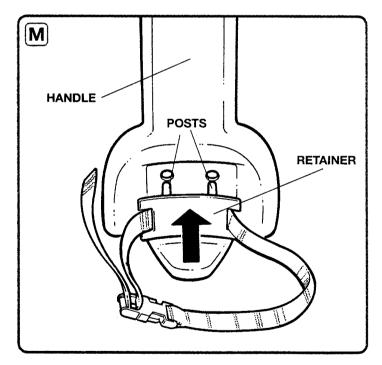
12. Insert posts on retainer into 2 holes in indentation on handle (the retainer correctly fits in the indentation only one way). (See Illus. M.)
