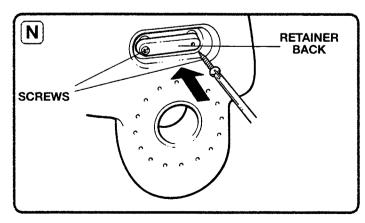
13. Holding retainer in place, turn handle over and place retainer back over retainer posts. Insert 2 screws into holes and tighten with Phillips screwdriver. Do not over-tighten screws. (See Illus. N.)
