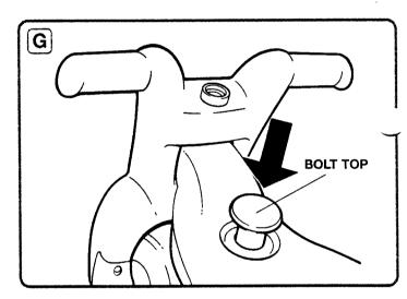
7. Turn toy right side up. Insert footrest bolt top (piece with flat top) into hole in body. (See Illus. G.)
