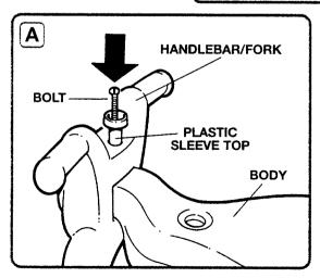
1. Slide handlebar/fork onto front of body. Align holes in top and bottom of andlebar/fork with holes in body. Insert plastic sleeve top into hole in top of handlebar/fork. Insert bolt into plastic sleeve. (See Illus. A.)
