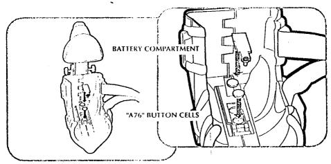
1.To replace batteries, hold skate with toe pointing upward. Use a Phillips screwdriver to loosen (but not remove) the screw that secures the battery door, and remove door. Remove used batteries and insert 2 new "A76" button cells in skate. Replace door, tighten screw with screwdriver, and repeat procedure with the second skate.
