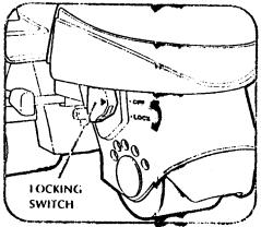
To lock front wheels in the conwird-only rolling position, turn the switch to the "LOCK" position. Wheels will not roll backward in this setting.
