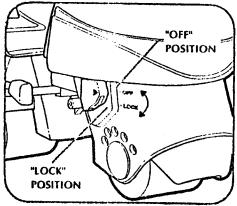
To return front wheels to the "free-wheeling" mode, turn the locking switch to the "OFF" position. Wheels will roll both forward and backward in this setting.
