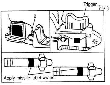
1. Apply labels to unassembled parts, using numbers on the label sheet and these illustrations as a guide.
