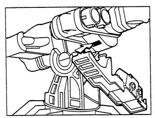
4. Hook sighting console into slot on lower part of gun.
