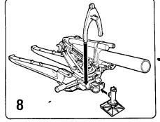
Snap base into chassis front end support arms as shown. Snap wishbone into front end of chassis.
