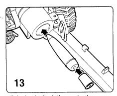
To load projectile shell, open chamber door and insert shell then blast cap. Close chamber door.
