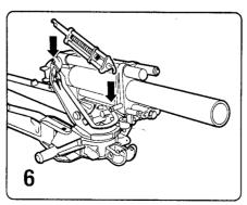
Snap right or left piston/spring onto cannon. Repeat for other piston/spring.
