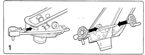
Snap crank case assembly into cannon support. Snap crank handle into crank case shaft as shown. Snap second crank handle into cannon support.
