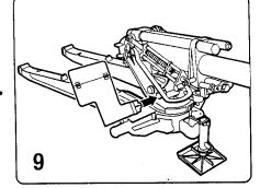
Snap right protective shield onto cannon support then repeat for left protective shield.
