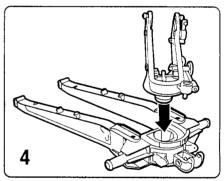
Snap cannon support into hole in chassis.
