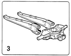
Snap right and left chassis legs into chassis as shown.
