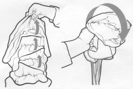
2. Starting at one end, gather each section of parachute together, one section at a time. Fold gathered parachute in half.
