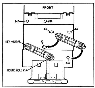
IMPORTANT: Assemble FRONT HINGES FIRST. FOLLOW STEP BY STEP WHEN ATTACHING BAY FLOOR HINGES.
