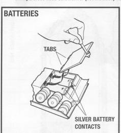
Place tank on side. Use a Phillips/crosshead screwdriver (not included) to loosen screw securing battery compartment door, and remove door (screw remains attached to door). Remove and discard batteries. Insert 2 x 1.5v "D"/LR20 alkaline batteries. To assure proper power supply to the motor, gently bend silver battery contacts of battery box cover so they make firmer contact with batteries. Replace battery door and tighten screw with screwdriver. See diagrams.
