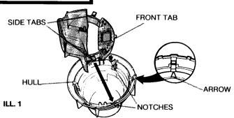
1. Line up tab on front of cockpit console with arrow on inside of hull. Fit side tabs into notches in hull. (ILL. 1)
