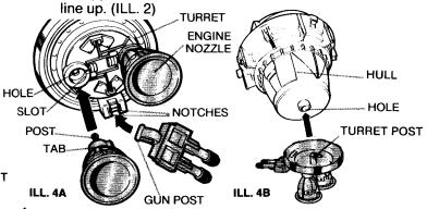
Line up tabs on engine nozzles with slots on turret. Snap nozzle posts into holes. With twisting motion, insert gun post into notches in turret. (ILL. 4A) Snap turret post into hole in bottom of hull. (ILL. 4B)
