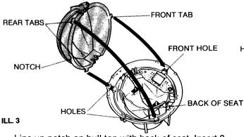
Line up notch on hull top with back of seat. Insert 2 rear tabs into holes in hull. Snap front tab into front hole. (ILL. 3)
