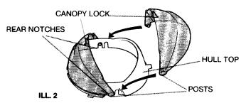
2. With canopy lock facing upward, fit posts into rear notches in hull top as shown. Repeat with second canopy and front notches. NOTE: Make sure locks
