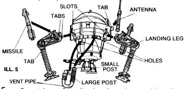
5. Snap tabs on 3 landing legs into slots on sides of hull. 6. Snap large post on vent pipe into hole on side of hull. Fit smaller post into hole as shown. Fit slot in antenna over tab on side of hull. Fit slots in 2 missiles over tabs on 2 landing legs. (ILL. 5)
