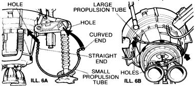
A. (Note: 3 small propulsion tubes attach to legs.) Insert CURVED end of small tube into hole on LEFT side of one landing leg. Bend tube and insert STRAIGHT end into hole in hull as shown. Repeat with remaining 2 small tubes and landing legs. (ILL, 6A) B. Insert ends of large propulsion tube into remaining
