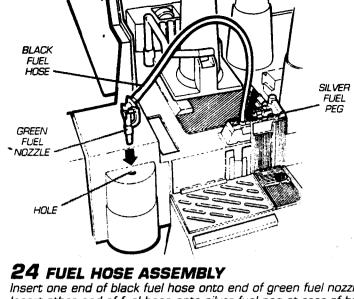
Insert one end of black fuel hose onto end of green fuel nozzle. Insert other end of fuel hose onto silver fuel peg at rear of base. To store nozzle, place into hole as shown.
