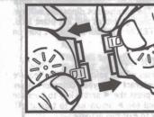
Press the locking tip and then pull the two units to release the Head-to-Head Connection.
