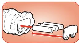
batteries. Replace cover and tighten screws.
