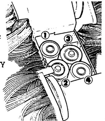
4. Insert edge of cover into side of compartment and swing cover down.
