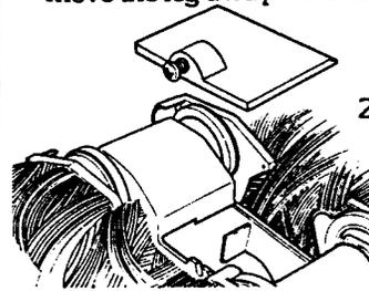
3. Insert 4 "D" size batteries in the order (1-4) shown in the illustration, and in the position (+ or -) shown inside the battery compartment.
