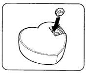
Discard used batteries and insert 2 new batteries, following direction indicators inside compartment.
