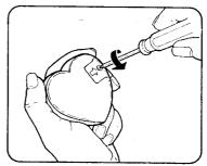
Loosen the small screw that secures the battery compartment door, and remove door.
