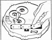
Place 3 size "C" Alkaline batteries inside the battery chamber.
