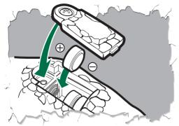
To Replace Batteries: Using a Phillips/crosshead screwdriver (not included), loosen screw in battery compartment cover. Remove cover. Remove and discard batteries. Insert 3 x 1.5v "A76" or LR44 size alkaline batteries. Replace door, and tighten screw with screwdriver. See diagrams for polarity.
