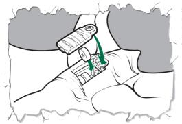
To Replace Batteries: Using a Phillips/crosshead screwdriver (not included), loosen screw in battery compartment cover. Remove cover. Remove and discard batteries. Insert 3 x 1.5v "A76" or LR44 size alkaline batteries. Replace cover, and tighten screw with screwdriver. See diagrams for polarity.
