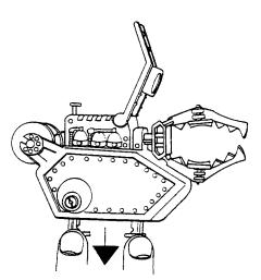
6. Sidecar has two legs that should be lowered when it is not attached to bike.
