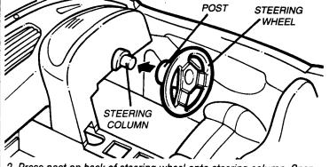
2. Press post on back of steering wheel onto steering column. Snap into place.
