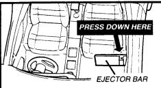
7. Press down on the ejector bar located in front of the passenger seat. Make sure you press the part of the bar that is closest to
