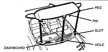
3. Align pins at center of windshield with holes on back of dashboard and snap into place. Align peg on one side of windshield to slot on same side of dashboard and snap into place. Repeat with other side.
