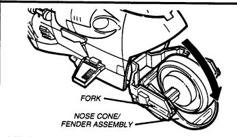
1. Hold vehicle right side up. Gently pull nose cone/fender assembly at front of sub until it drops into fork. Snap into position.
