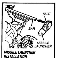
3. Slide slot on missile launcher
