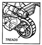
3. Turn vehicle around and swing turbo-props together. Align treads and snap into place as shown.
