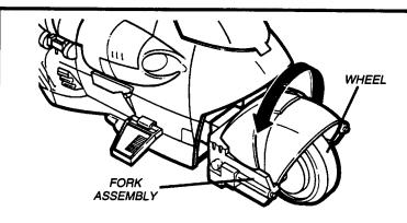
2. Rotate whole fork assembly about 180° until wheel "clicks" into position as shown.
