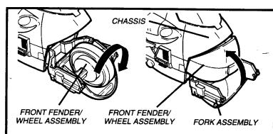
2. Rotate fork on front fender/wheel assembly so that wheel is facing upwards. Unsnap front fender/wheel assembly from fork assembly, swing into chassis and lock into place as shown.
