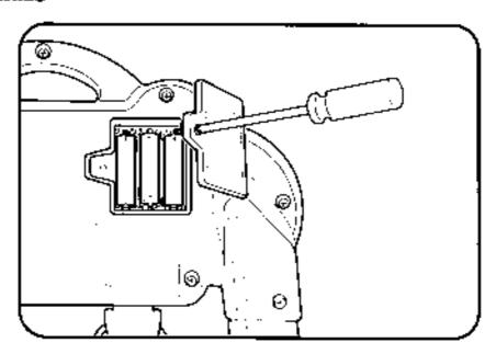
With Phillips screwdriver, loosen screw in battery compartment door on back of electronic housing (screw will remain attached to door). Remove door. Insert 3 fresh "AA" alkaline batteries into compartment. Replace door and tighten screw with screwdriver.
