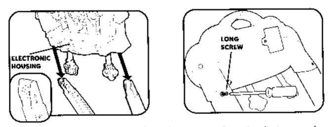
Turn assembly right side up. Stide electronic housing onto arms. Secure housing to arms using 2 long screws and Phillips screwdriver.
