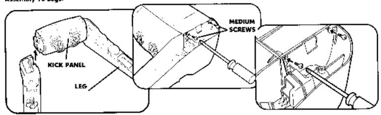
Attach kick panel to legs. Turn assembly upside down and place on flat surface. Using 4 medium screws and Phillips screwdriver, secure kick panel to legs.
